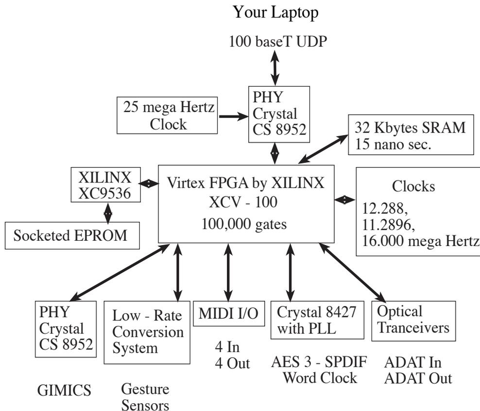
We have developed a VHDL module which implements Fast Ethernet from the hardware layer up through IP to the UDP protocol of TCP/IP. This unusual module is of particular value in our application because Fast Ethernet ports are available on all modern laptops. Also, because of the commercial importance of Internet performance, Fast Ethernet implementations are extremely reliable and finely tuned on all modern operating systems.
