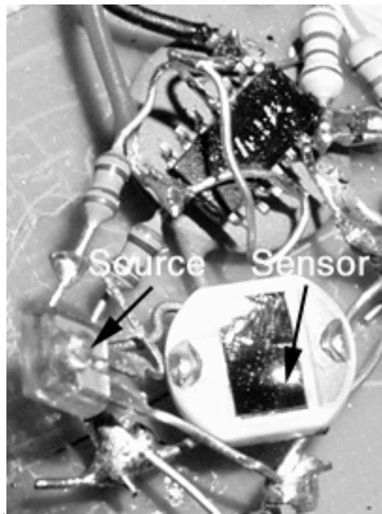
A reflection-based sensor operates by sensing light reflected from a source on the top plate below the string. Our preliminary work on this strategy revealed so many problems that we abandoned this approach in favor of the methods described below.
