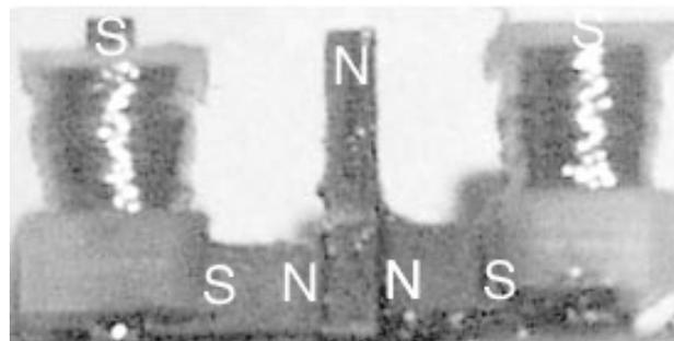
The pickup uses two coils around pole pieces of the same polar organization. Between these coils is a third pole piece of opposite polarity resulting in a two-ring field pattern with common flux lines at the center.
