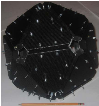
Figure 10. Pentagonal access holes at the vertices
