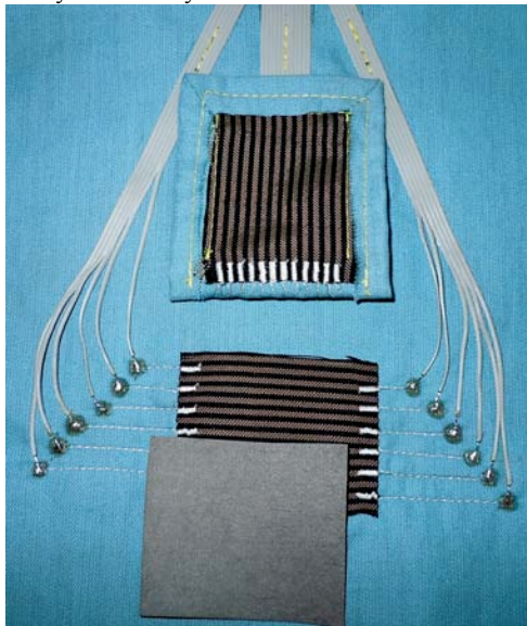
Figure 1: Strain-relieved cabling and solder pad
