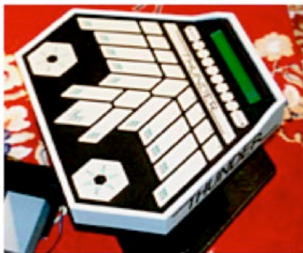
Figure 1: Thunder by Don Buchla. The ridge-separated strips are sensitive to both location and finger pressure. It sends MIDI controller data and is both continuous and polyphonic in character.
